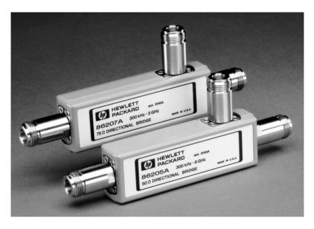
The HP 86205A/86207A high directivity RF Bridges offer unparalleled performance in a variety of general purpose applications. They are ideal for accurate reflection measurements and signal-leveling applications. They combine the directivity and broad-band frequency range of directional bridges and the low insertion loss and flat coupling factor of directional couplers.
